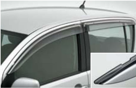
2 Door visor for cold weather pack 08610K1002 Allows windows to stay open for ventilation during unsettled weather. With an incision to prevent the door hinge from freezing when parked at night in cold areas.
