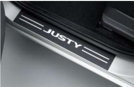
17 Side sill plate J105EFD200 E Protects the side sill plates from damage when getting in and out of the car. Finished in a stylish aluminium tone, these serve as an ideal highlight for the step.
