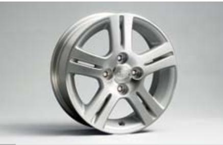
11 Aluminium alloy wheel (14 inch) 42611B1030 14x5JJ offset 40 175/65R14
