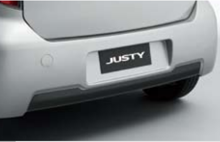
7 Rear bumper lower styling foil E775EFD300 Stylish black foil which also helps protect lower part of rear bumper from scratches.
