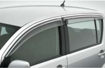
1 Door visor 08610K1001 Allows windows to stay open for ventilation during unsettled weather.
