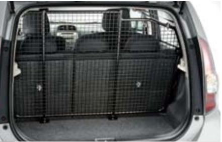
27 Dog guard F55SEFD000 E Separates cargo room from passenger area, applicable for ISOFIX child seat.
